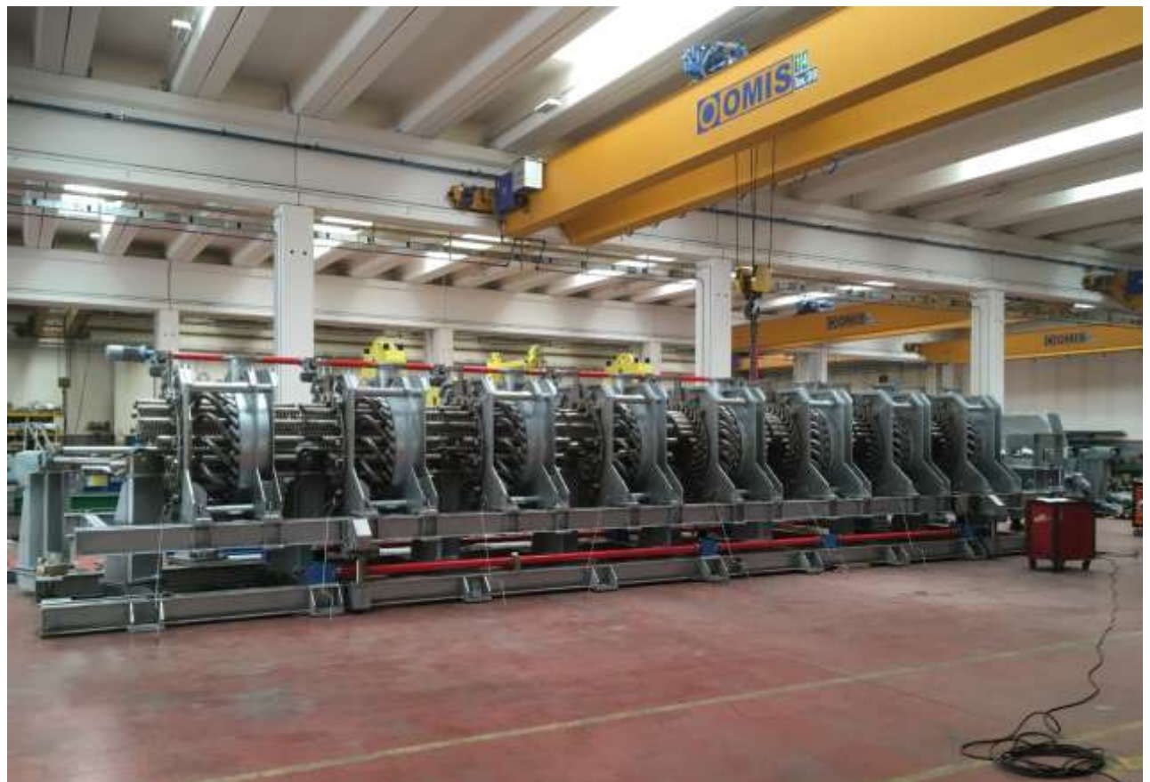
Descalers and quenching heads for tubes hardening – built as per customer’s patented engineering
