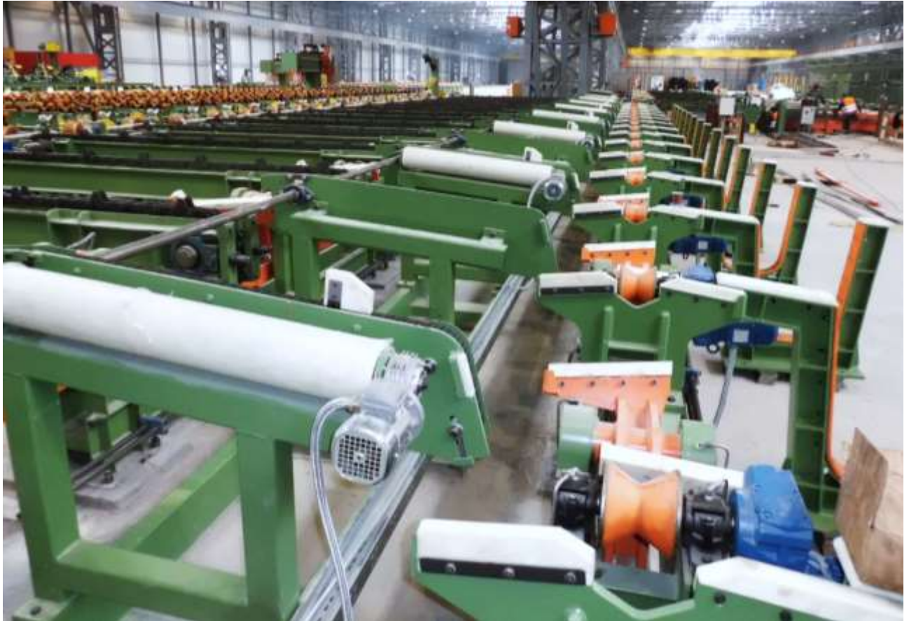
Ends tube brushing machine station
