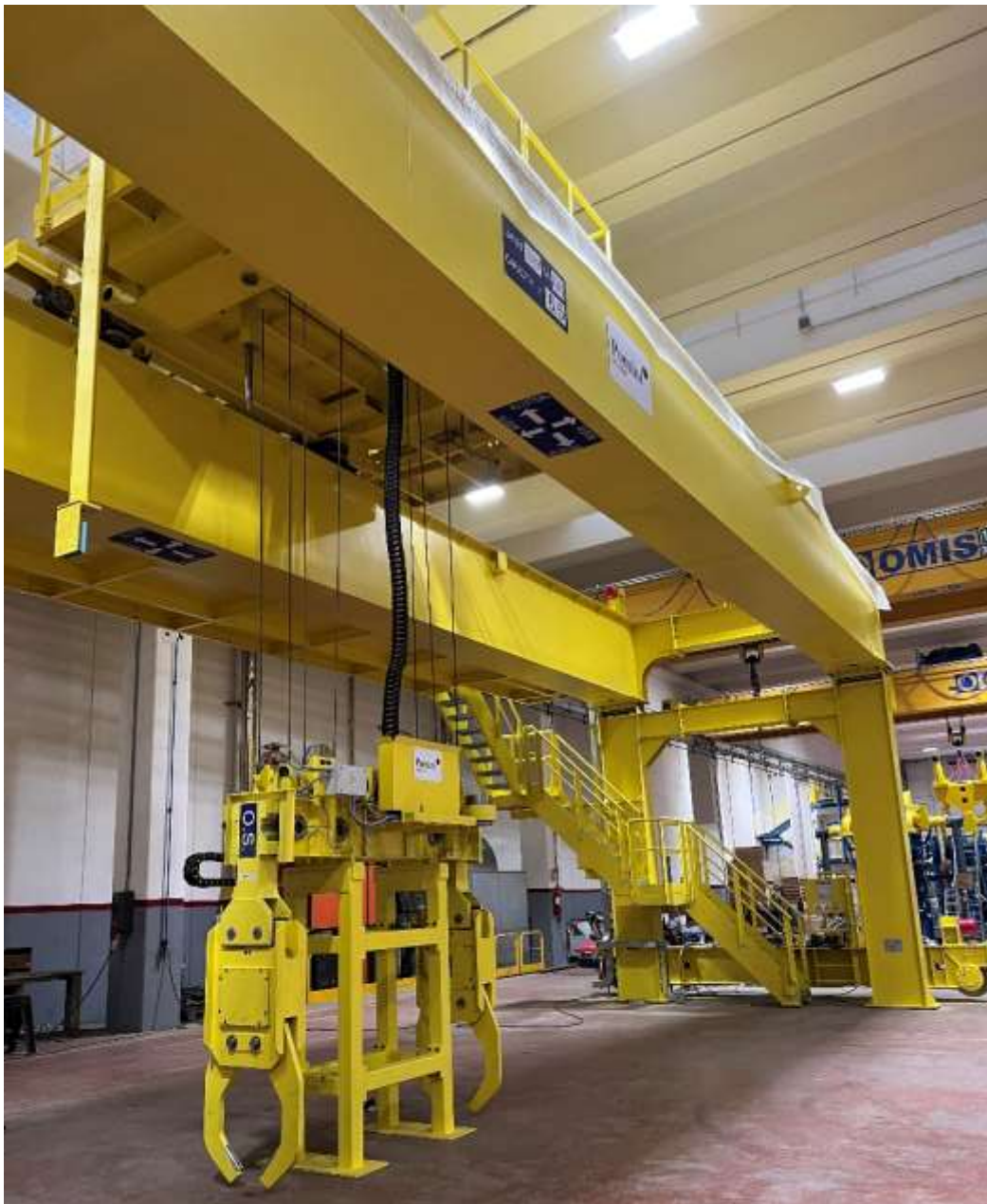
Gantry and tongs for work rolls
