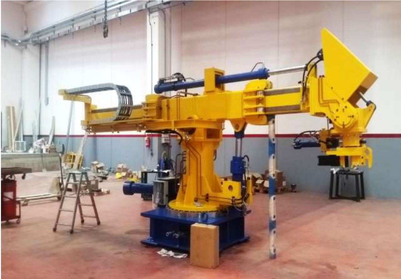
Rod Manipulator for coil opening - built as per customer's engineering
