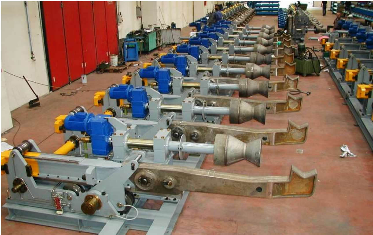
Electric pipes extractor from hardening furnace
