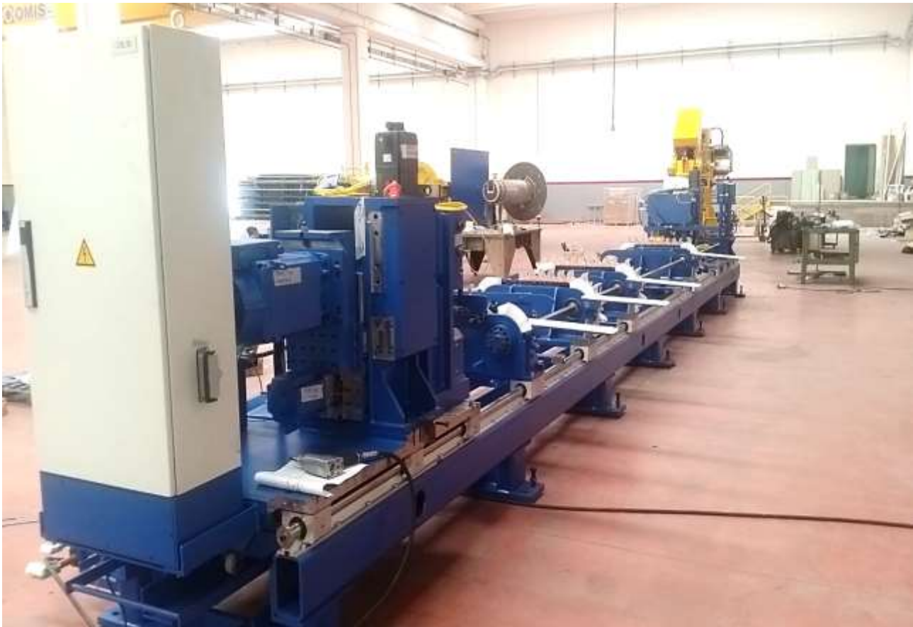
Chamfering machine for bars - built as per customer's engineering
