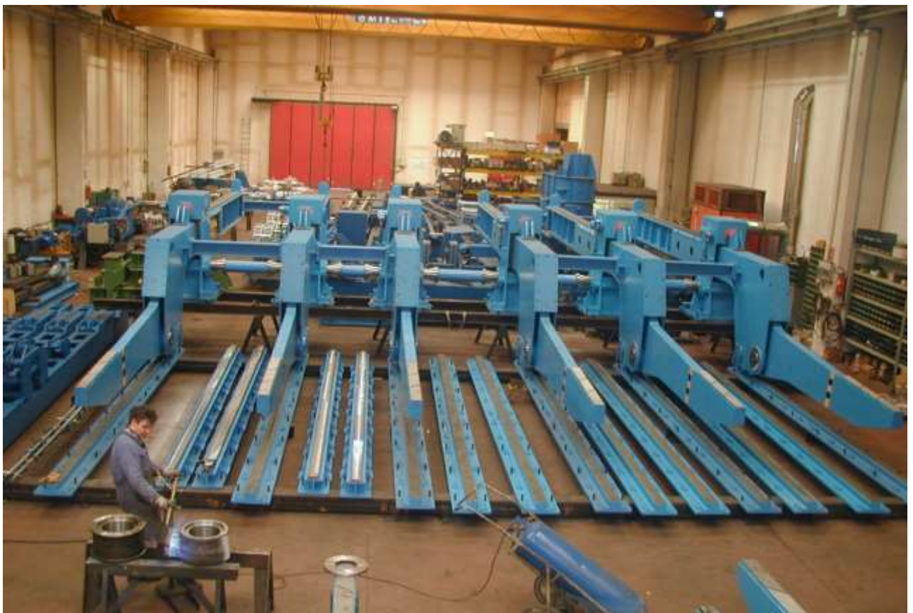
Reheating furnace charging and discharging devices for slabs
