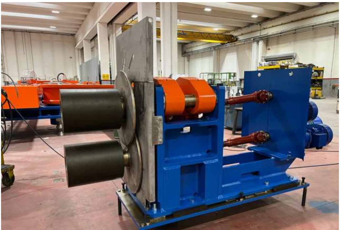
Hot billes discharging Pinch roll
