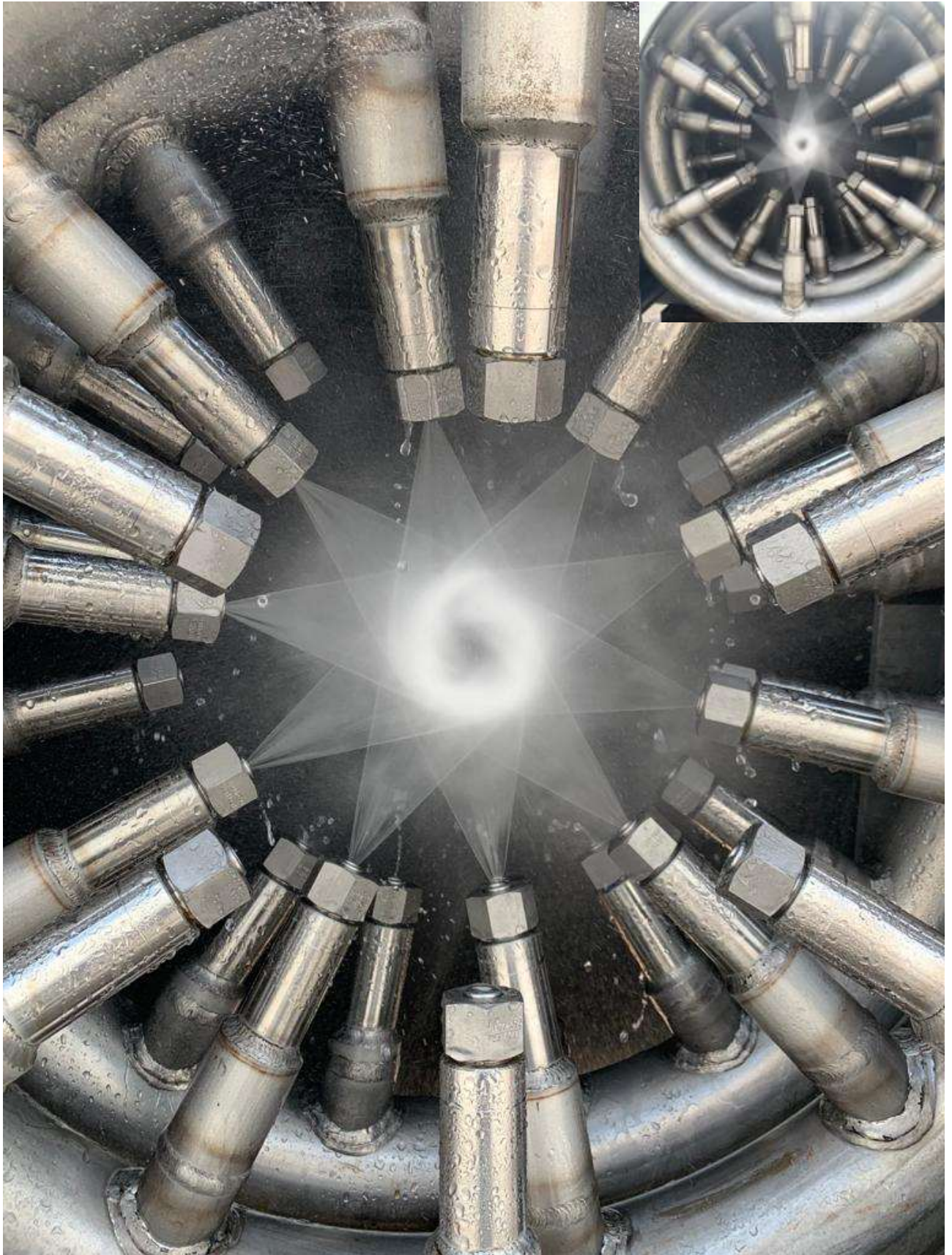
Testing phases for descaler head
