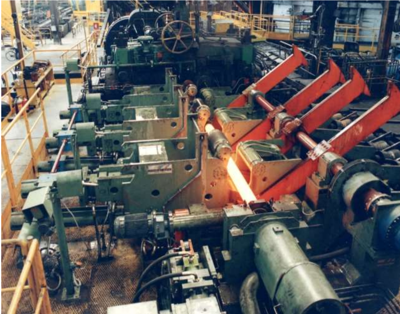
3-roller self-centring guides for tubes piercing mill
