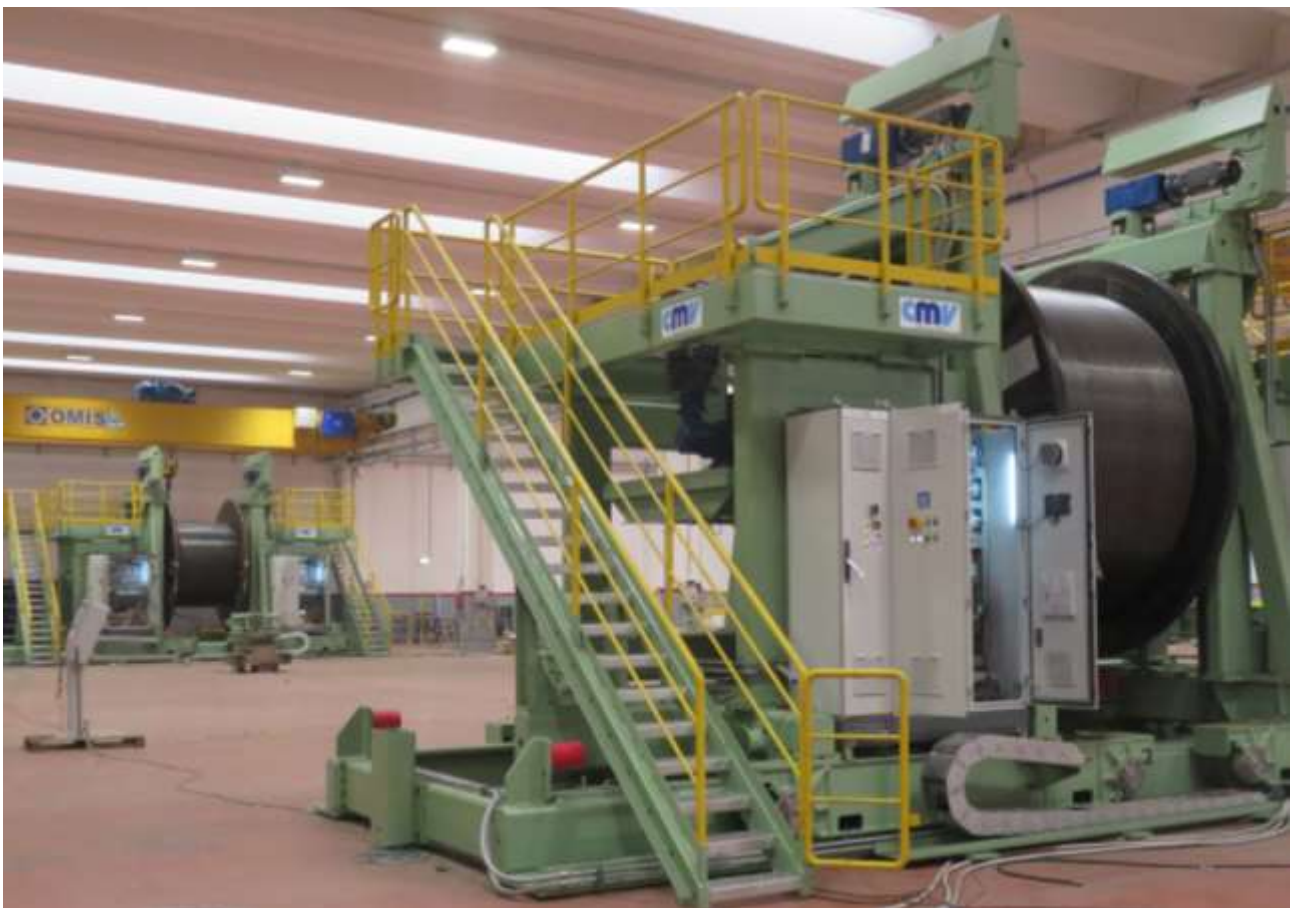
Spoolers for tube laying (CMV's entire engineering)
