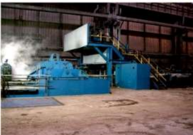
Revamping of shear and roller ways for strip mill
