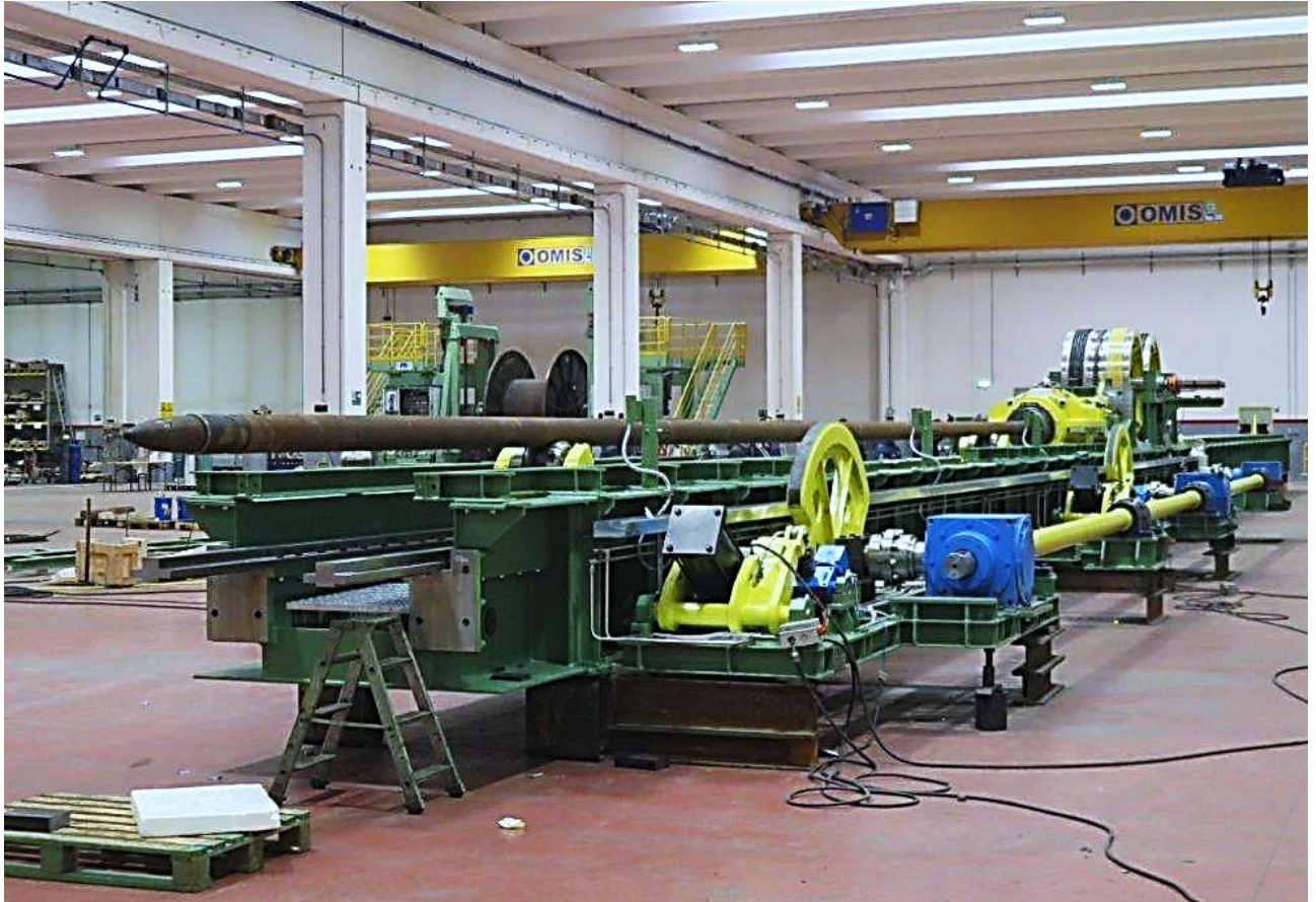
Piercer fast chuck trolley (6 m/s speed)
