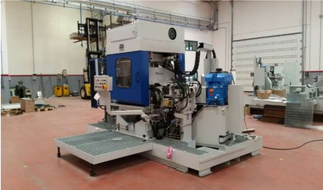
Two-Roll Straightener for round bars - built as per customer's engineering
