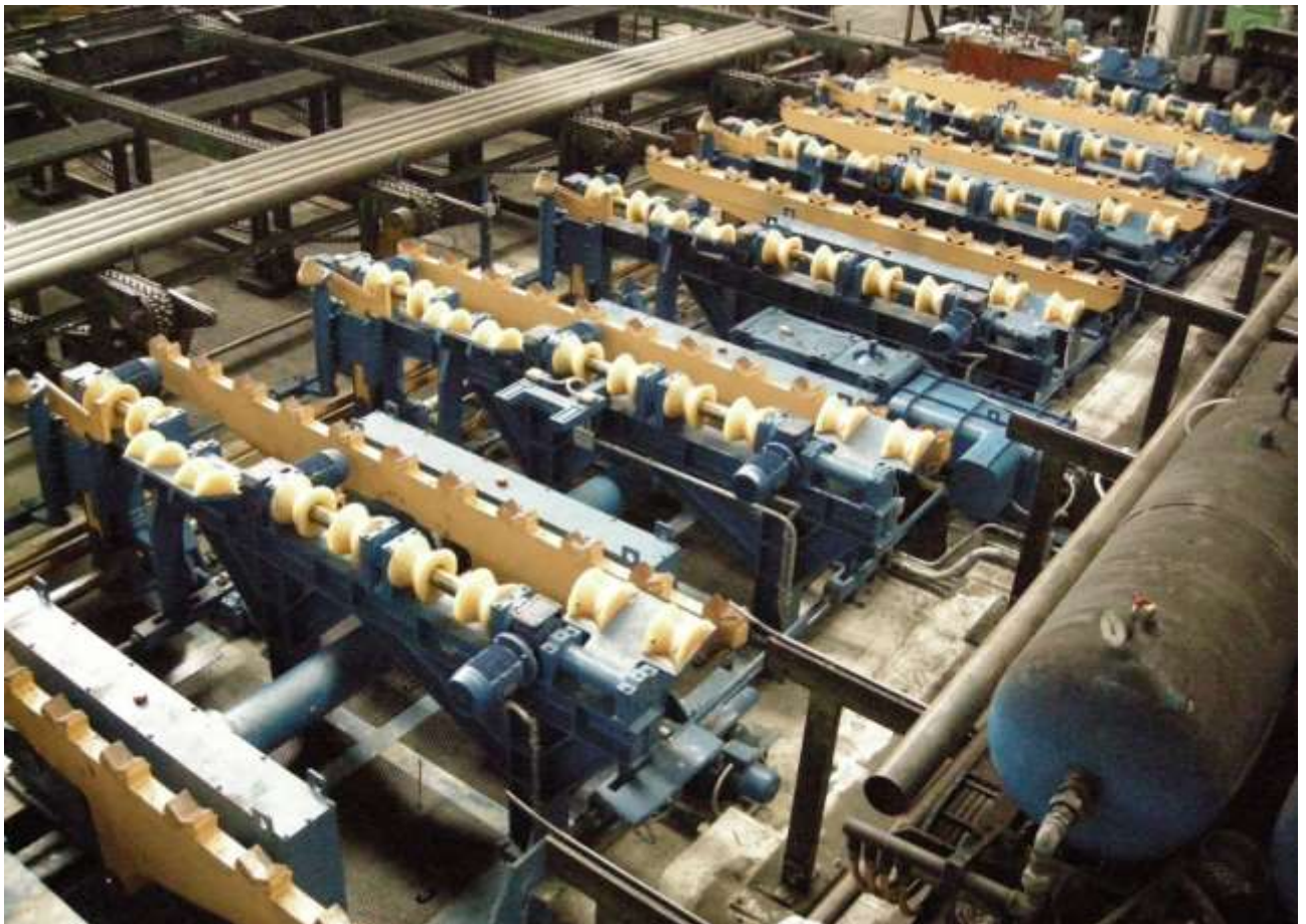
Walking beam for tube chamfering machine (cycle time 1 s)
