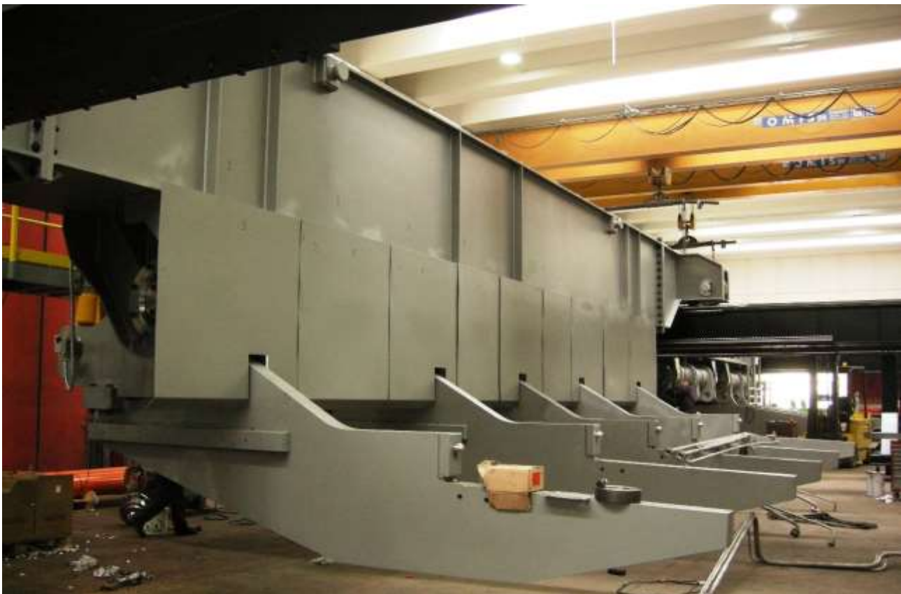
Slab discharging device from reheating furnace
