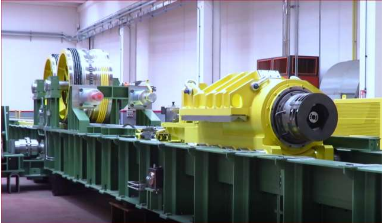
Piercer fast chuck trolley (6 m/s speed)
