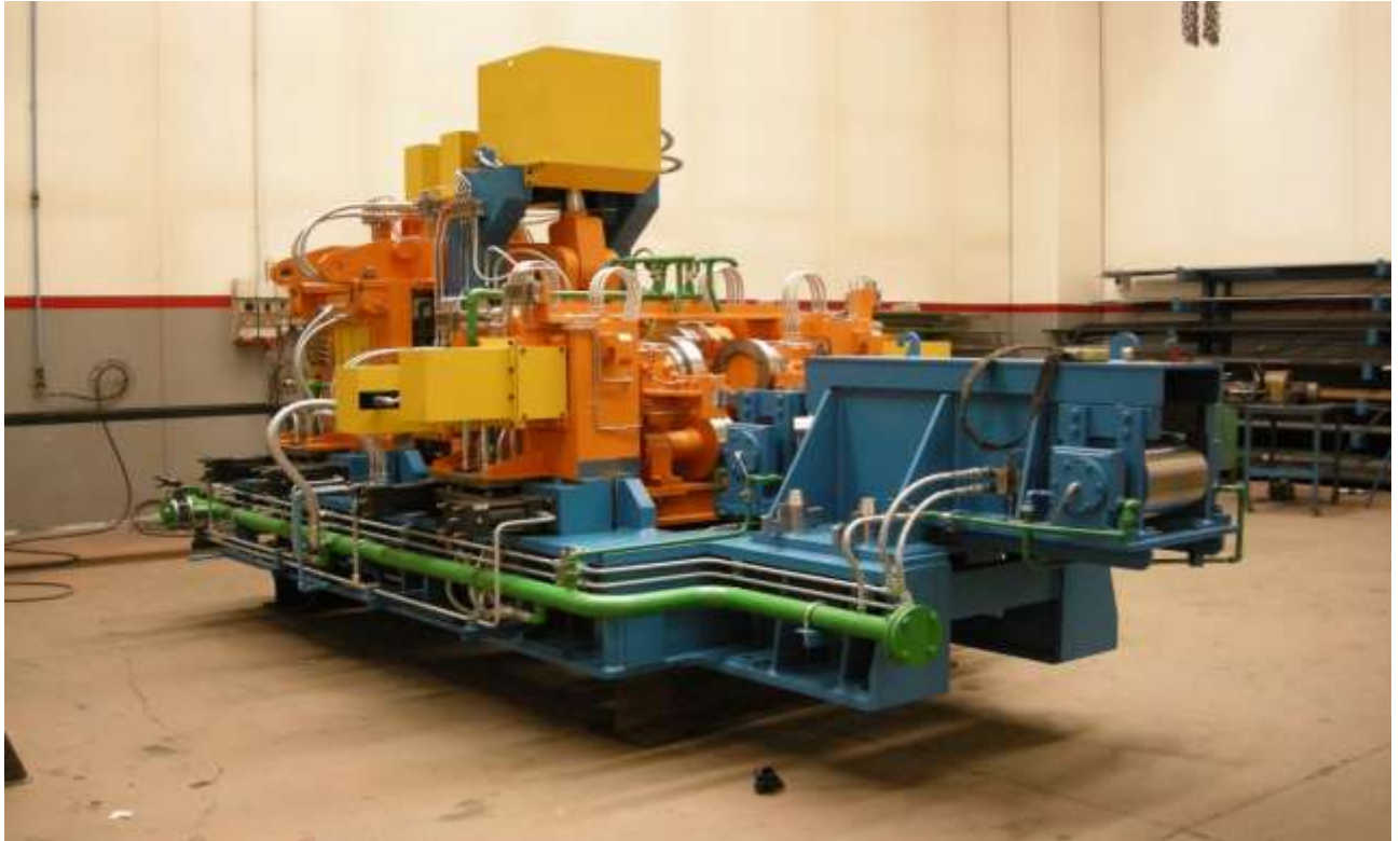
Deburring machine for hot-welded billets - built as per customer's engineering
