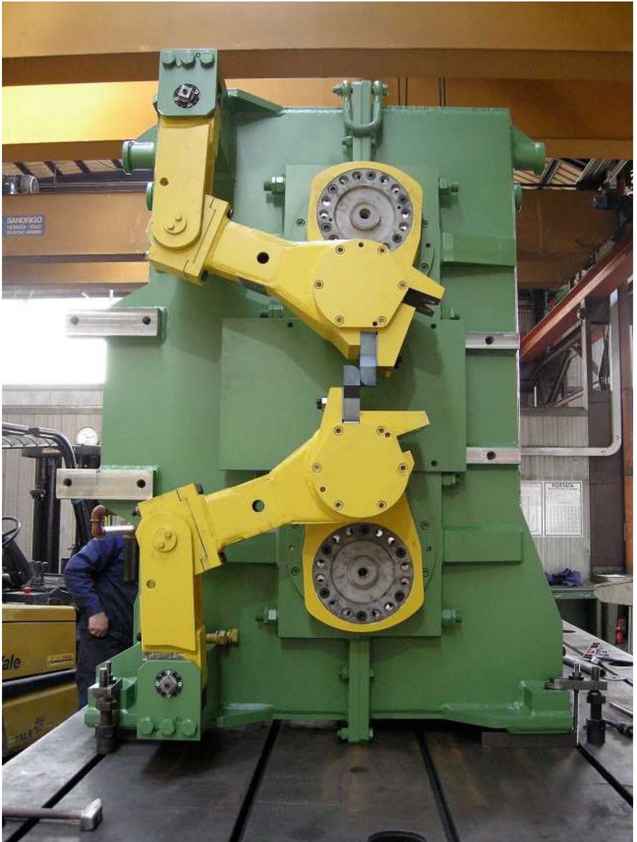
Start-stop shear - built as per customer's engineering
