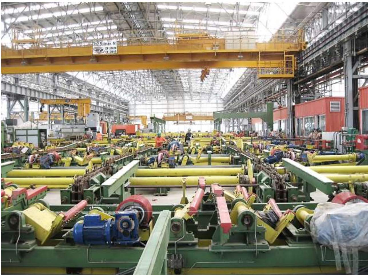
Handling on complete tube finishing line OCTG diam. 114 / 400 mm
