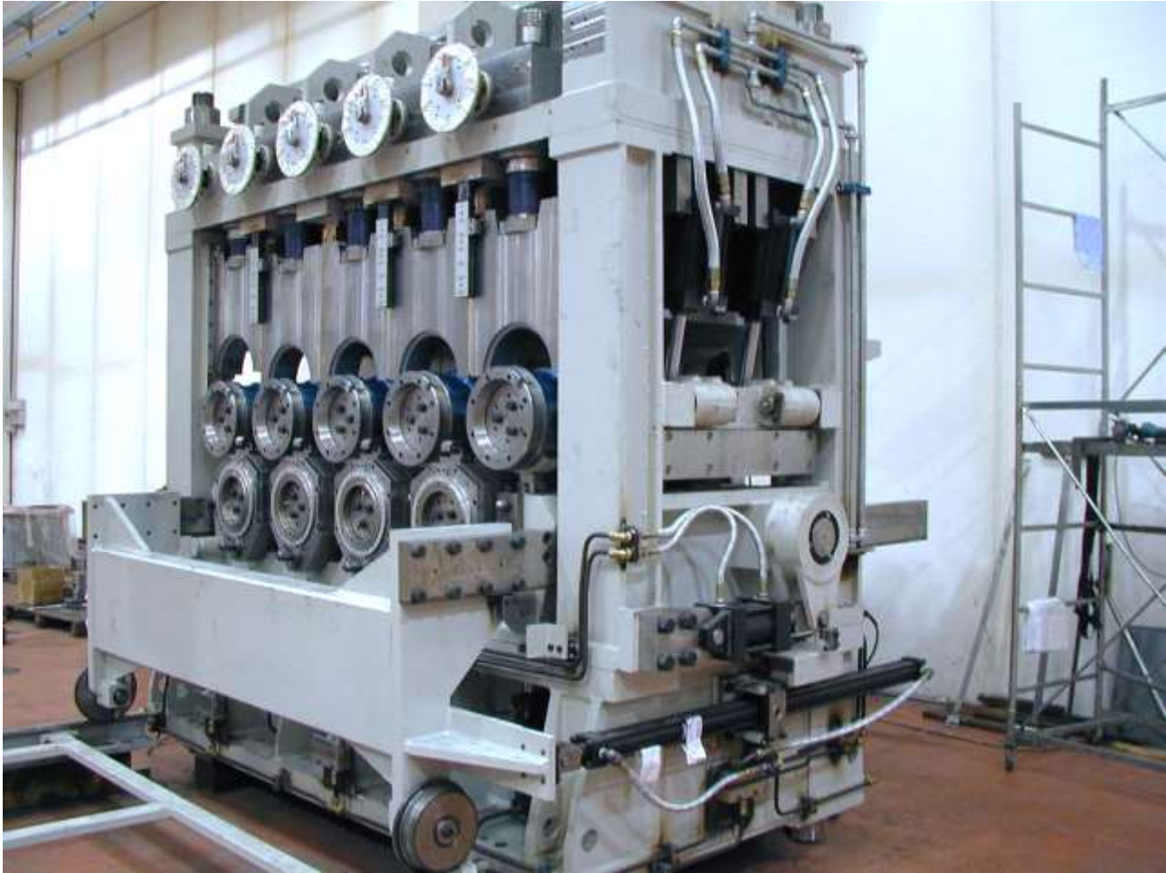
Hot profiles straightener – built as per customer’s engineering
