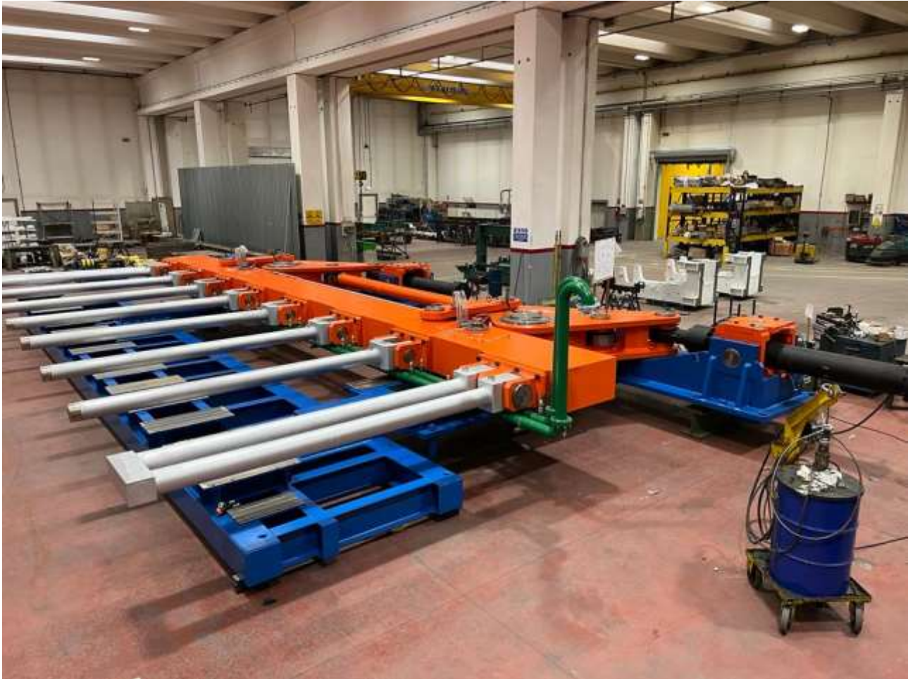
Charging pushers for billets reheating furnace
