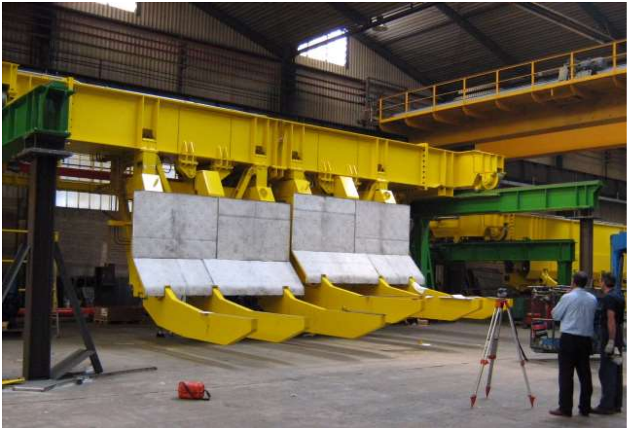
Slab discharging device from reheating furnace
