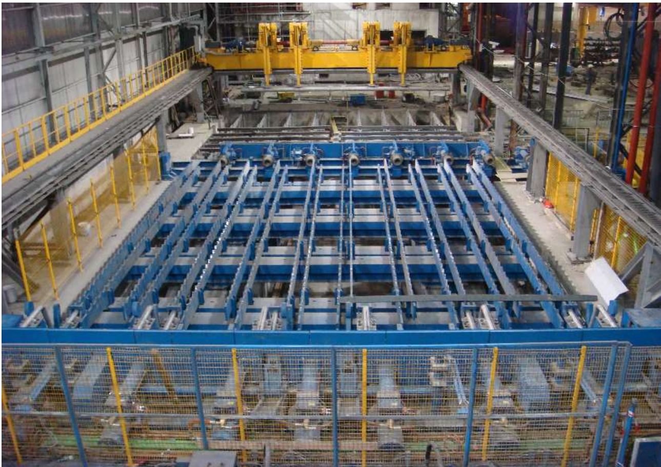
Direct charge of billets from continuous casting machine to reheating furnace
